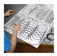
Our O-ring flip charts are an easy way to help determine what size O-ring you have. Simply move your O-ring over various image outlines to find the right size that matches. This chart includes sizes from O-ring series O, 1, 2, 3, 4, as well as O-rings for tube fitting bosses.
